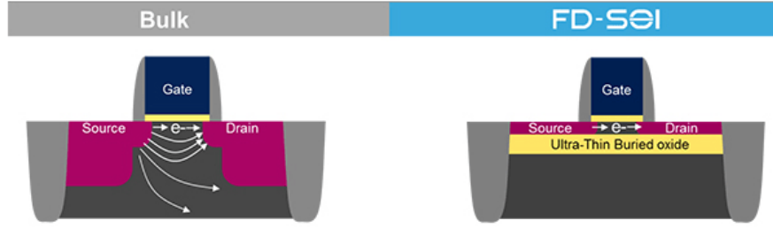
Fig. 2.1: Bulk based MOSFET vs FDSOI based MOSFET [2]
