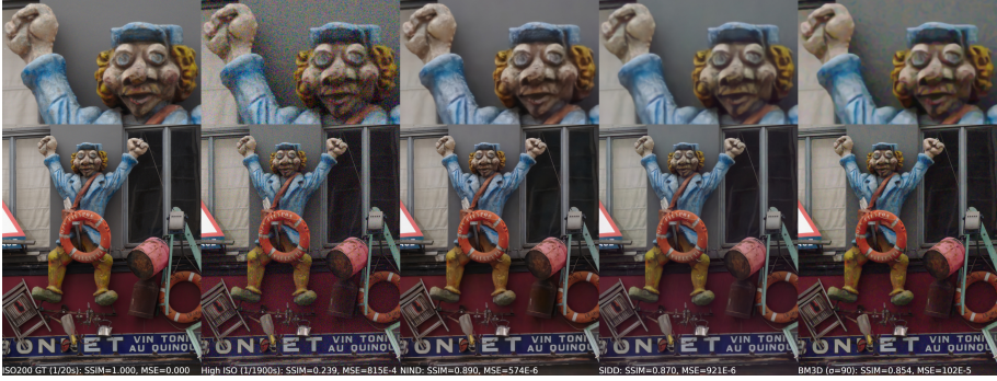
Figure 2.5: Denoising results on the “stefantiek” test image from NIND. From left to right: 1: ISO200 ground-truth (s.s.: 1/20 s), 2: high ISO (s.s.: 1/1900 s), 3: 2 denoised using a U-Net model trained with NIND, 4: 2 denoised using a U-Net model trained with SIDD (320 image pairs), 5: 2 denoised using BM3D ( \sigma = 90 ).
