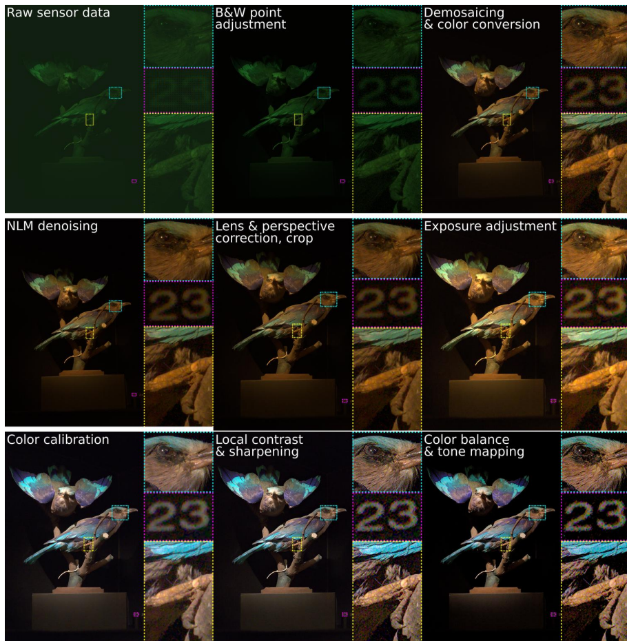
Figure 5.1: An image development pipeline illustrated using Darktable 5.0 and a moderately noisy image (taken at ISO16000). Throughout this work, we refer to stage 1 as the Bayer input, stage 2 as the Linear RGB input, and stage 8 as the developed image (although NLM denoising is shown in step 3 for illustrative purposes, prior denoising is not applied in the development pipeline for the developed images used as input to the models in this work, as shown in Figure 5.5.) Darktable was chosen as our primary tool for raw image development due to its wide use within the photography community and its open-source nature, ensuring transparency and reproducible experiments.
