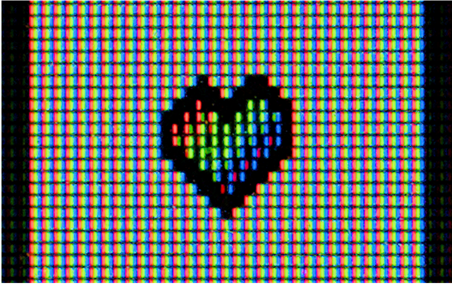
Figure 2.1: Close-up photograph of an LCD display showing a grid of pixels with their individual RGB components (sub-pixels).
