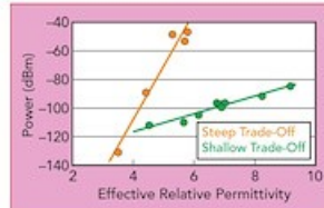
▲ Fig. 7 Second harmonic vs. \epsilon for porosification setups yielding steep and shallow trade-offs.
