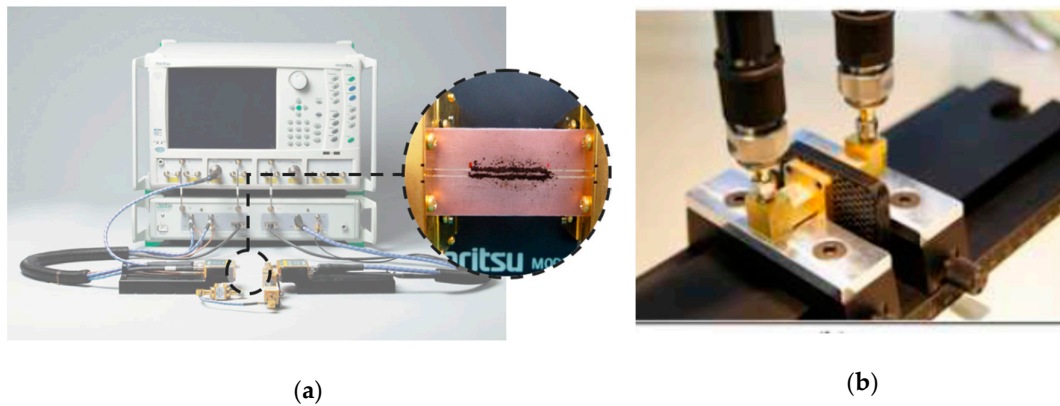
Figure 3. (a) Measurement configuration for nanoinclusions powders (b) measurement configuration for absorber thin plates, adapted from [23].
