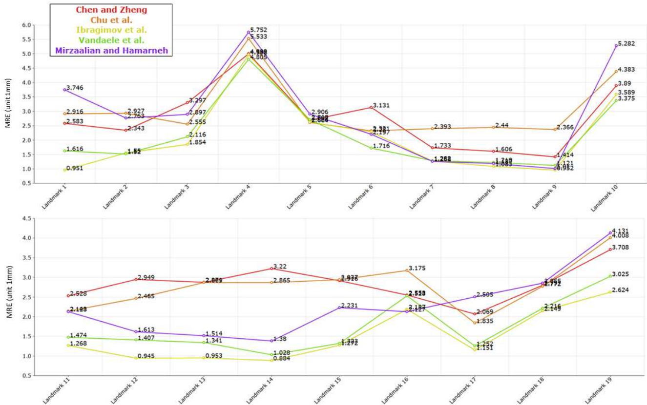
Fig. 10. Mean radial errors (MREs) with 1 mm as the measurement unit in detection of individual landmarks on Test1 data. MREs for Landmark 4, Landmark 10 and Landmark 19 are particularly high, showing that these landmarks are especially difficult for detection.
