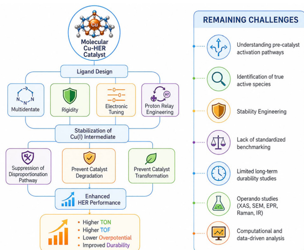
Fig. 25 Schematic representation of emerging design principles, key challenges, and future research priorities for molecular copper HER catalysts.
