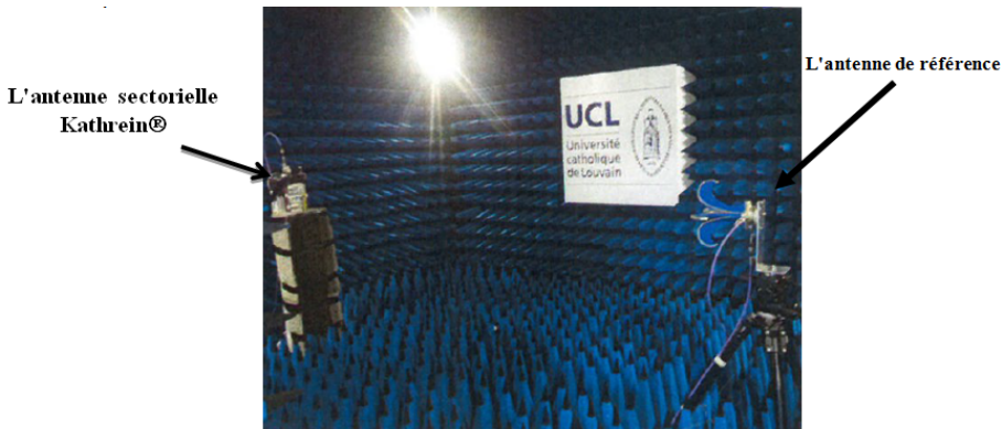
Figure 9.4: GSM Antenna measurement setup
