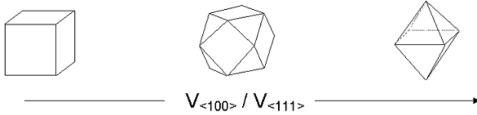
Figure 2.5: The variation of the crystal morphology with the ratio of the growth rates along \langle 100 \rangle and \langle 111 \rangle directions [19].
