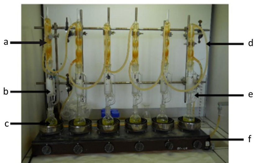
Figure 3.13: Lipid extraction in Soxhlet apparatus. Butterflies were placed in paper filter bags in a cartridge (b); Diethyl ether was warmed up (f) in a balloon (c) and evaporated; it cooled down in the condenser (a) cooled by running water (d) and sank back in the balloon with the overflow system (e). Picture: C. Marchand.
