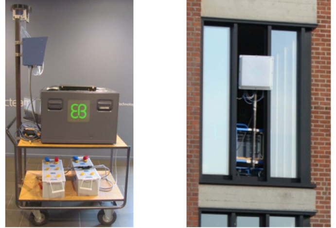
Fig. 1. Photo of the BS and the MS used for the measurement campaign. Left: MS. Right: BS.
