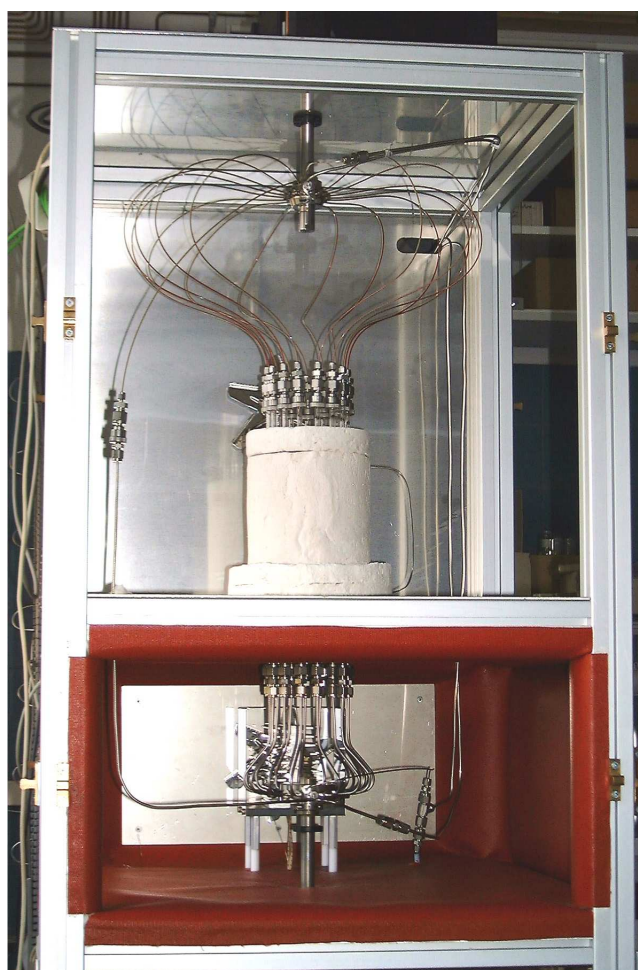
Figure E-1: 15-channel reactor used for carrying the metathesis reaction.
