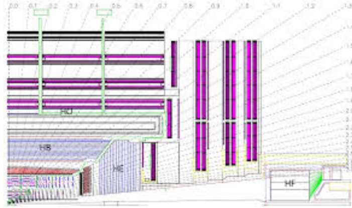
Figure 2.7: Transverse view of one quarter of the CMS HCAL with pseudo-rapidity benchmarks shown as dashed lines.
