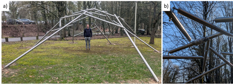
Fig. 2. The RS-24B prototype, built outdoors: a) General view and b) Central rings.
