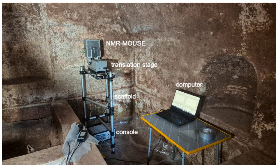
Fig. 2. NMR setup for measuring depth profiles. The NMR-MOUSE is mounted on a precision translation stage, which rests on an adjustable scaffold. The sensor and the translation stage are connected to the console, which is operated by the computer.
