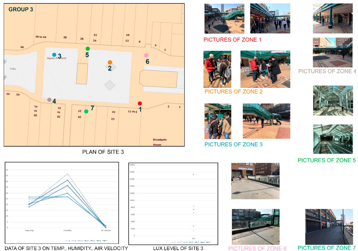
Figure 1. An example of a student project to explore outdoor thermal comfort. Master of architecture students used questionnaires and data loggers in the city centre of Coventry, UK.
