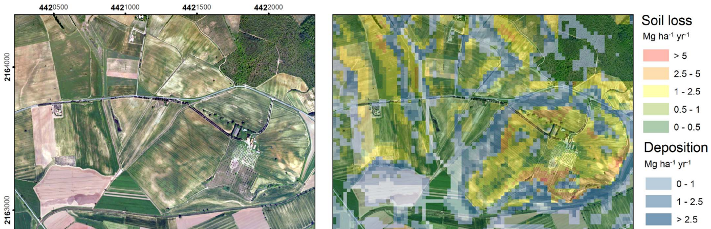
Fig. 4. WaTEM/SEDEM results in hilly arable lands ongoing soil erosion and degradation processes in the Southern Tuscany (Magliano, 4421500 N – 2163500E).
