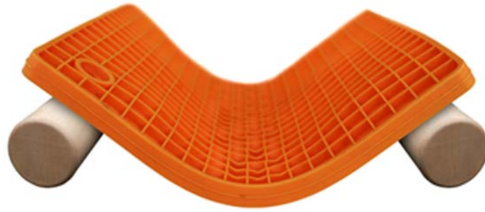
Figure 10. Loading condition for the pot mat.
