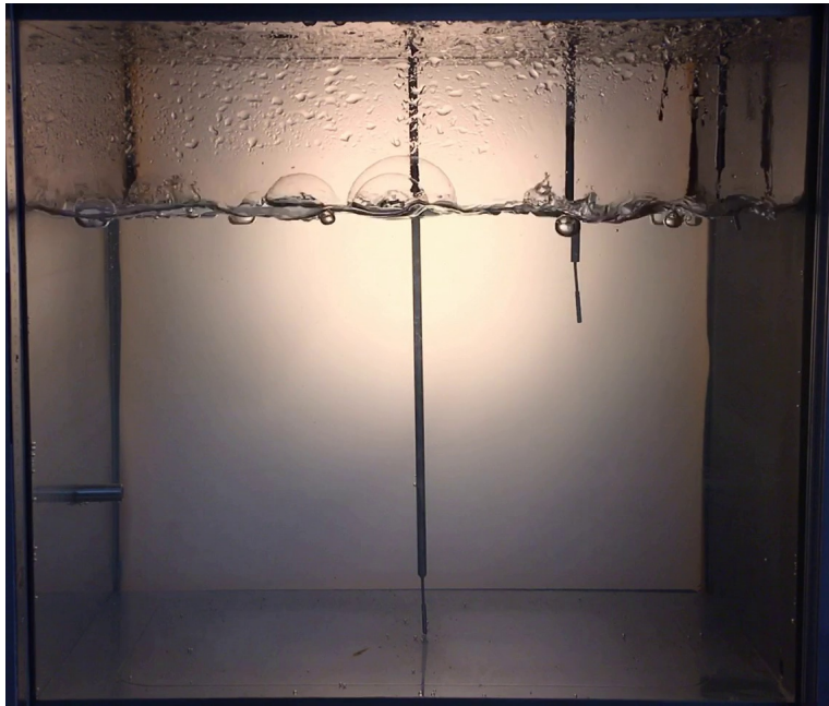
Figure 8. During the first stage of the test and after the initial strong bubbling originating from the immersed walls, the superheated water continuously flashed and turned into bubbles just below the liquid free surface.
