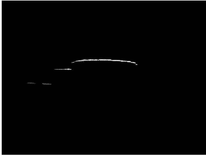
Fig. 5.10. Typical image after elimination of the objects with a low height-to-width ratio.
