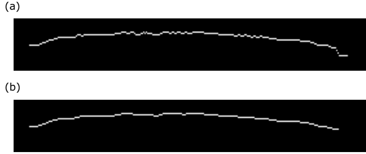
Fig. 5.17. Laser curve on the reference image (a) before and (b) after smoothing.
