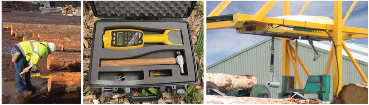
Figure 6. Left: Measuring with the Hitman HM220, middle: the Hitman HM220, Right: Sawmill use of the Hitman LG640.
