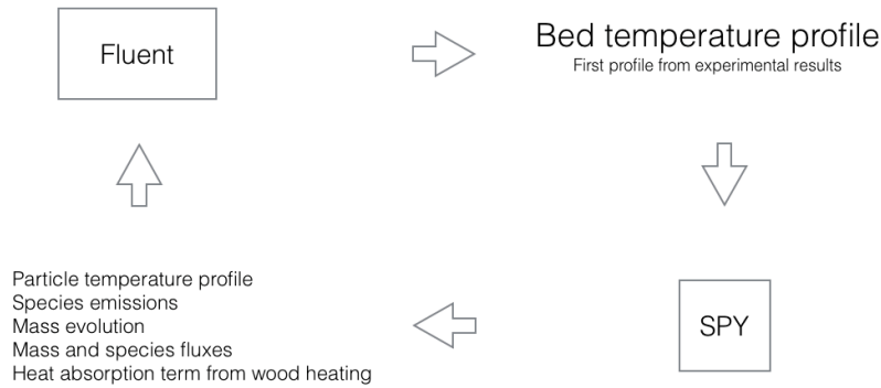
Figure 5.7 – Illustration of the coupling of SPY and Fluent ® .
