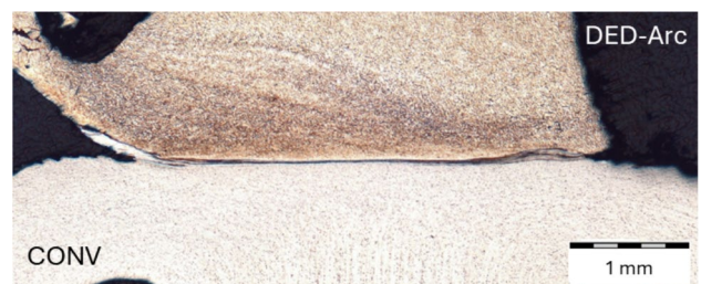
Fig. 15 Incomplete joining region in the RFW weld of conventionally manufactured EN AW-5083 to DED-Arc manufactured ER 5183 parts
