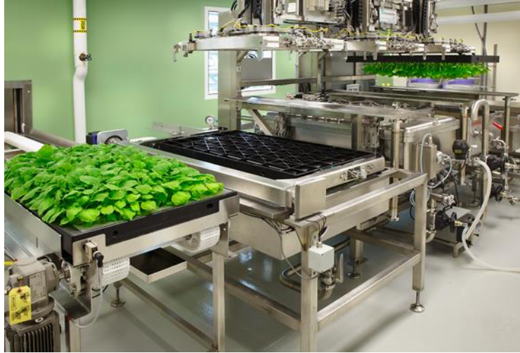
Figure 1. N. benthamiana vacuum infiltration unit (Fraunhofer USA). When the N. benthamiana plants are about 12 cm tall, the rack is placed upside down into a container containing an Agrobacterium culture. A vacuum is applied and all the air in the plant is pulled out. When the vacuum is turned off, the interstitial spaces are filled with Agrobacterium , which will transform the cells.
