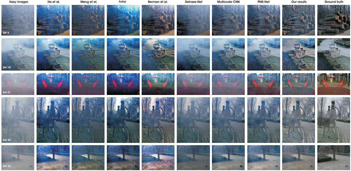
Fig. 2. Qualitative comparison of dehazing methods [3], [6], [4], [5], [8], [7], [31] and our method for 5 images of the O-HAZE dataset.
