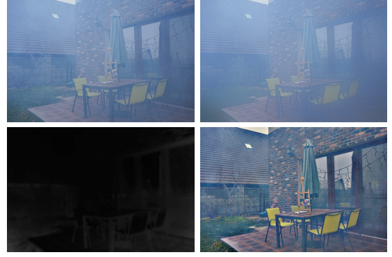
Fig. 1. Considering the hazy image (top-left), our refined airlight estimate \bar{A}_\infty (top-right) shows a similar appearance with the original hazy image (since we basically filter out from the hazy image only few high frequencies). Using our zero-close transmission (Eq. 3) (bottom-left) we can solve the optical model and generate our dehazed result (bottom-right).
