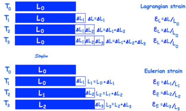
Figure 13 Lagrangian strain (top) and Eulerian strain (bottom). Lagrangian strain is the sum of all length increments up to that time divided by the baseline length, while Eulerian strain at any time is calculated as the sum of all ratios of length increments and the instantaneous length up to the actual time.
