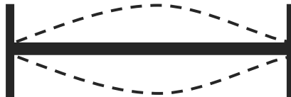
Figure 57, (a) Vibration of a fixed-fixed beam at its fundamental mode (b) with possible adjustable mass
