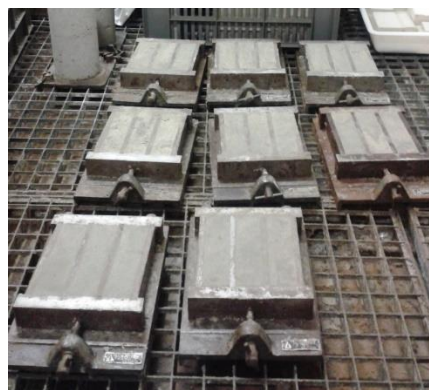
Figure 27, Specimens placed in the moist room
