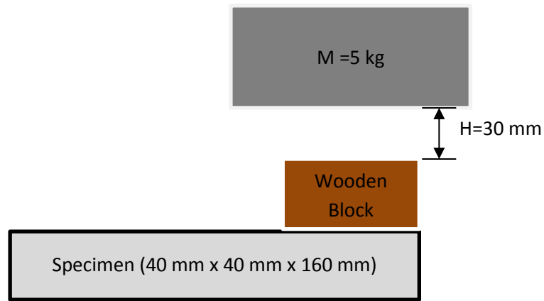
Figure 26 Schematic illustration of compaction process
