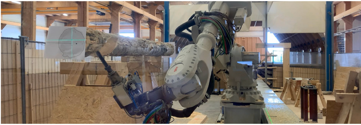
Fig. 39. Milling of a timber log with a 6 DoF robotic arm (from the authors, 2020, videos on: [54,55]).
