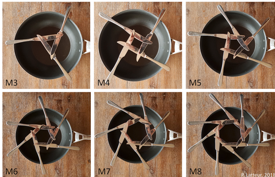
Fig. 7. Basic reciprocal moduli with varying beam quantities.
