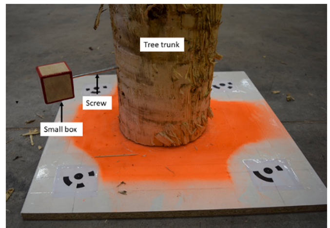
Fig. 17. To define the Y and Z axes, a long screw with a small 60 mm box at one end of each trunk is placed, large enough to be modelled photogrammetrically.
