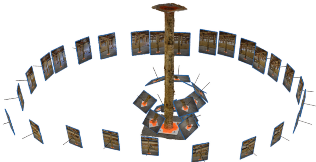
Fig. 16. Orientations of photos taken for 3D scan with photogrammetry, taken with a Nikon D5300 using a Nikon AF-S DX NIKKOR 18–55 mm f/3.5–5.6G VR II camera lens.
