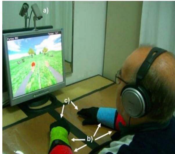
Figure 9b. The Rehabilitation Gaming System: tracking through camera with data gloves [53].
