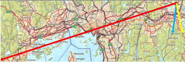
Fig. 2. Path trough first 2.5 km of atmosphere towards Inmarsat-5 F2 (39 km) in red, Astra 3B (6.5 km) in yellow and Ka-Sat (6.3 km) in blue.
