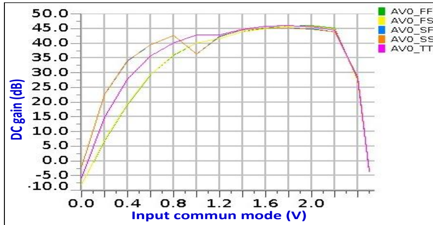
Figure 5.43: Simulated DC gain of the hardened OTA of Fig.5.41, for the different process and TID effects versus the input common mode, at T=200^{\circ}\text{C} .
