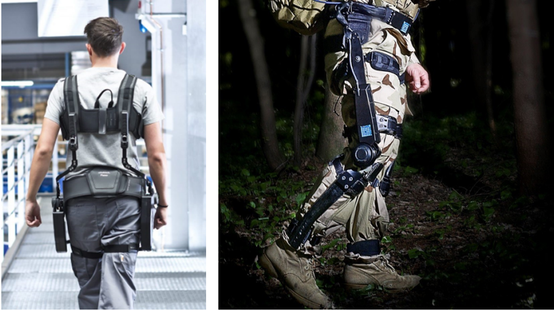
Figure 1.3: Typical exoskeletons designed for supporting healthy people to perform heavy duty tasks such as lifting or traversing over various terrains and carrying heavy equipments [19, 20].
