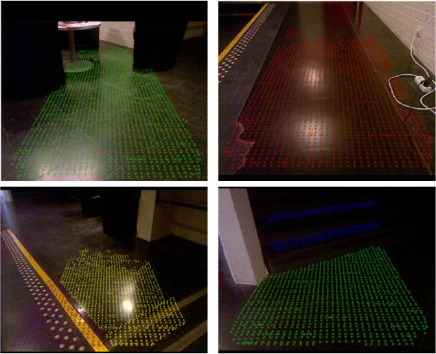
Figure 3.8: Detection samples of five locomotion captured with Kinect sensor in real environment. The point cloud for each terrain type are colored labeled with the labels given in Table 3.1.
