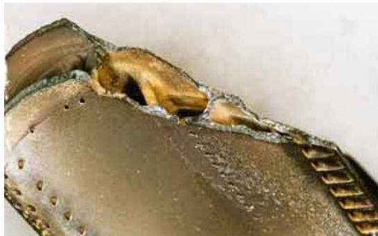
Figure 1-7: Material loss at the blade tip due to high heat transfer coefficients generated by the leakage flows across the tip (General Electric rotor blade)
