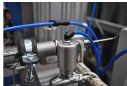
Figure C.17: Thermocouple-capteur de pression.
