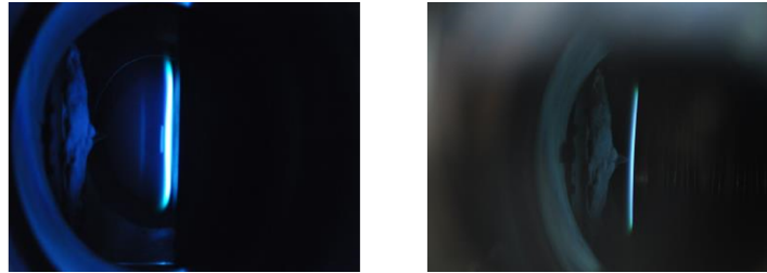
Figure 2.21: Picture of rich ethyl valerate flame at 20 mm (left) far from the quartz nozzle: burned gases and 3 mm (right) near the quartz nozzle: reaction zone.
