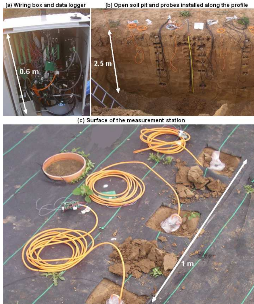
Figure 2.9. Picture of the installation phase of an experimental plot (summit position): (a) all soil probes are connected to a wiring box with multiplexer, dataloggers and batteries; (b) a soil pit has been dug until c. 2.5 meters depth to allow probes installation (i.e. for soil moisture and temperature); (c) after filling the pit, the surface of the measurement station is covered by a geotextile, collars for surface CO 2 fluxes are installed, and probes for profile CO 2 measurements are inserted vertically.
