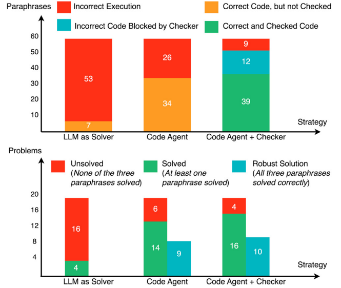
Fig. 4. Ablation study on the performance of the LLM-based agents. Top: performance across all paraphrases ((20 problems) \times (3 paraphrases) for each). Bottom: performance over all 20 problems in the test set.
