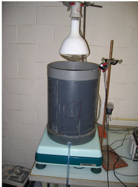
Figure 3.3. Experimental set-up of the lysimeter experiment.
