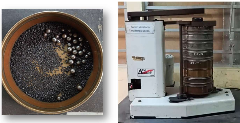
Fig. E. 1: Left: Hardness test pan with carbon and steel balls. Right: mechanical sieve-shaker with tapping hammer
