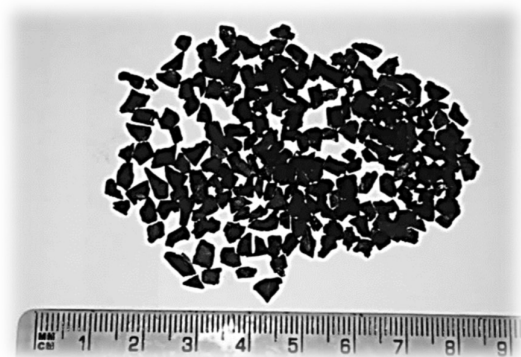
Fig. 1. 5: Granular activated carbon, Calgon, GR 20-22
