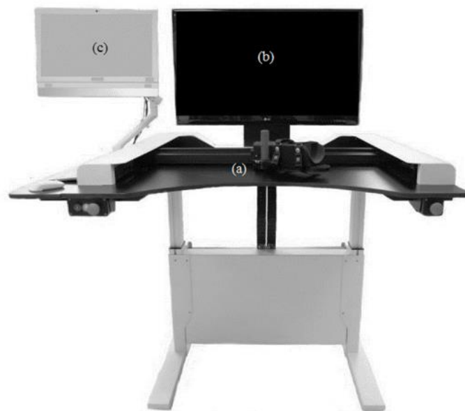
Figure 1. The REAplan ® end-effector robot (permission to use image allowed from Axinesis; Copyright), with: (a) a handle for interaction that measures position and force, (b) a visual interface for the participant, and (c) a visual interface for the experimenter / clinician.
