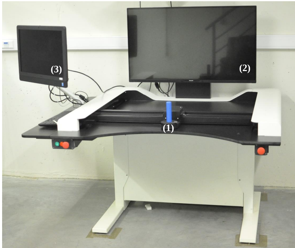
Figure 1. The REAplan ® robotic device. The device incorporates: (1) an end-effector with position and force sensors, (2) a monitor for the participant and, (3) a monitor for the experimenter.
