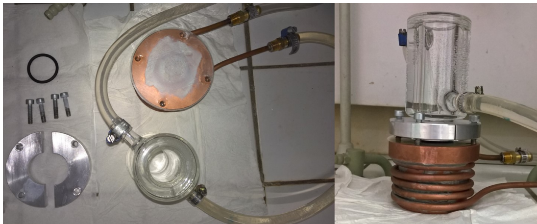
Figure A.1: Pictures of the large anodization cell, disassembled and assembled.
