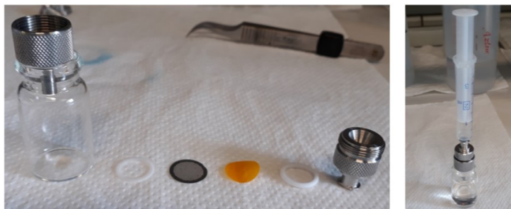
Figure 7.3: Picture of the material used for filtration on a PI membrane.
