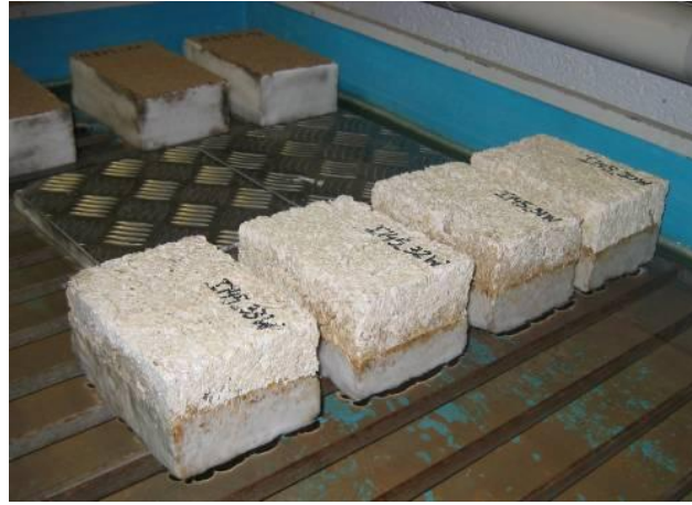
Figure 83 : Water absorption coefficient measurement
