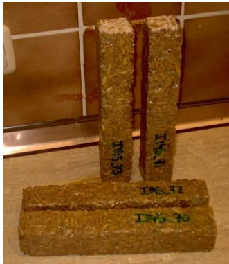
Figure 86 : Sample used in NMR apparatus
