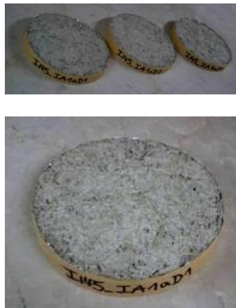
Figure 33 : LHM-wall (Barvaux's hemp)
