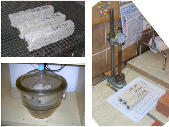
Figure 73 : Measuring swelling of LHM-wall
