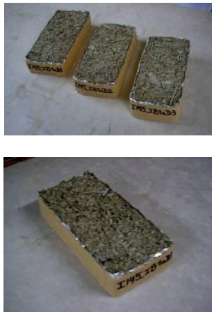
Figure 32 : LHM-roof (Barvaux's hemp)
