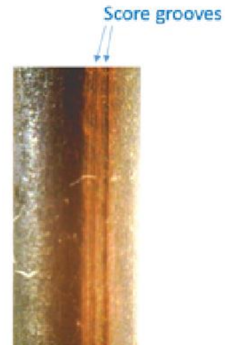
Dig- scope view of an 1880 iron wire nail showing the external dressing marks. Author.
