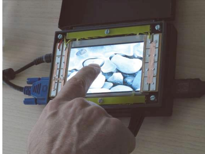
Figure 4. Interaction with a transparent touch screen with haptic feedback. Friction is modulated through piezoelectric actuators located on the frame of the device. Adapted from Giraud et al. 2012.
