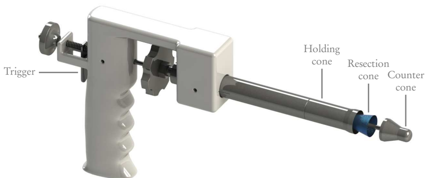
Figure 10.7: Solidworks modelling of the new version of the demonstrator.
