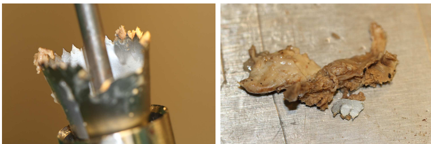
Figure 10.2: Because of the muscles contraction due to the embalming process and of the design of the blade, a too high effort was applied on the resection cone resulting in its fracture.
