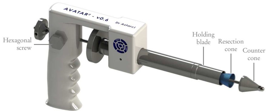
Figure 10.1: Solidworks modelling of the new version of the demonstrator.
