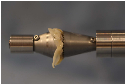
Figure 8.10: Leaflet placed between the resection cone and the counter cone.
