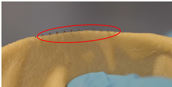
Figure 8.6: Results of the piercing of the bovine pericardium. Encircled in red, teeth of the blade that passed through the tissue sample.
