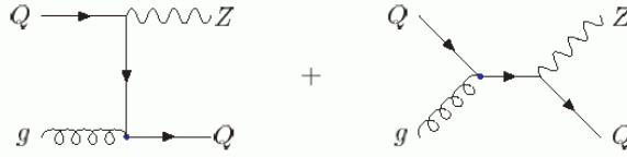
Fig. 2: Leading Order Feynman diagrams for associated production of a Z boson and a single high- p_T heavy quark ( Q = c, b ).
