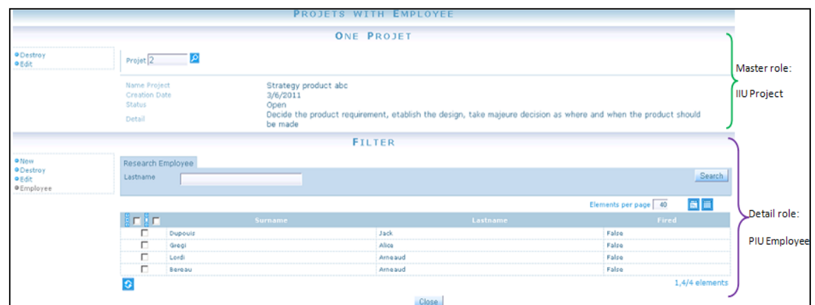
Fig. 7.3 Master-Detail pattern for a Web application
