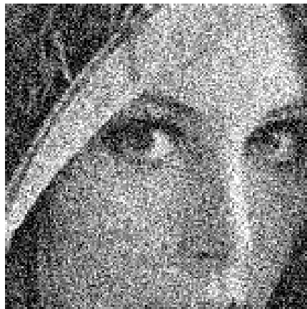
(b) Lena image with additive gaussian noise \sigma_{noise} = 40
