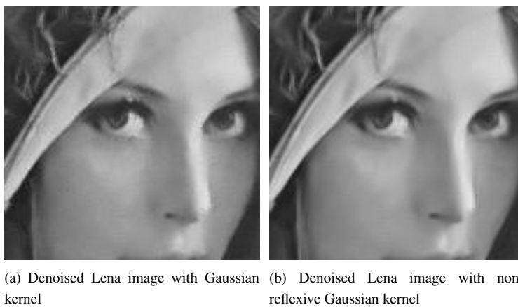
Figure 4.5: Examples of results obtained for the Lena image with \sigma_{\text{noise}} = 20 .
