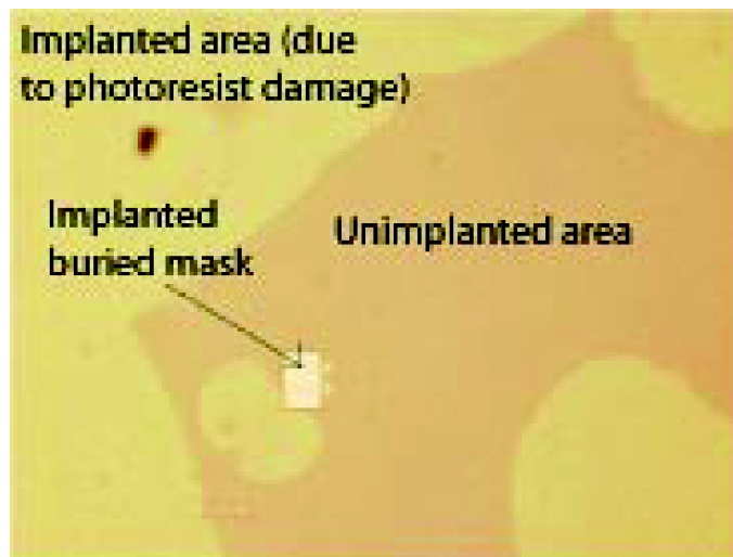
Figure 3.17: Optical microscopy of the sample surface after photoresist removal. The dark zones are the one that were protected by the photoresist mask. The light zones are the one where the resist was destructed.
