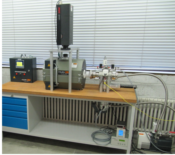
Figure 2.15: Photograph of the annealing setup. Center: Vacuum chamber and furnace. Upper part: multi-beam optical sensor. Left part: furnace control panel. Right and lower right parts: vacuum pumps and gas inlets.
