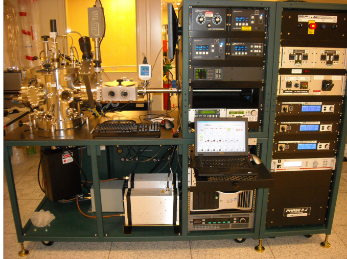
Figure 2.6: Photograph of the sputtering setup. Upper left part: vacuum chambers. Lower left part: multi-beam optical sensor. Right part: control panels.
