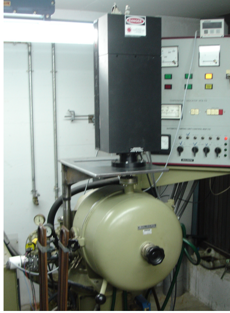
Figure 2.11: Photograph of the hydriding setup. Upper part: multi-beam optical sensor and vacuum/gas inlet control panel. Lower part: Vacuum chamber.
