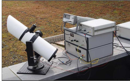
Figure 1.6: The LASEF system with the LASER source and the telescope on the left.
