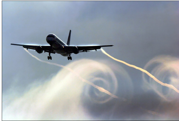
Figure 1.1: Illustration of the wake vortex phenomenon from a Boeing 757-2B7 flying through clouds. The aircraft is descending through 200 m about one minute from landing with full landing flap 30 selected to increase its lift coefficient and fly safely at lower speeds. In this configuration, the wake vortices are principally issued from the flaps. Courtesy of Steve Morris, from www.airliners.net .
