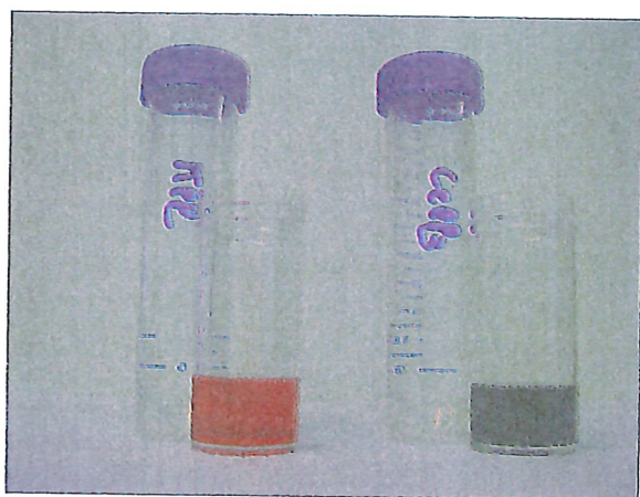
FIG. 1.12. – Suspensions of gold colloids bearing citrate groups at their surface, after the addition of a few drops of (left) a KCl solution, (right) a \text{CeCl}_3 solution. The purple-blue suspension obtained after adding \text{CeCl}_3 becomes transparent, with a blackish deposit, after a few hours, while the red suspension obtained in presence of KCl is stable. This experiment was performed based on reference [8].
