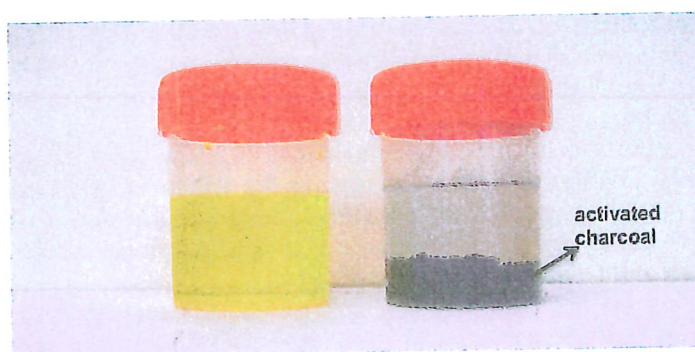
FIG. 1.1. – Solution of a yellow food dye, before (left) and after (right) treatment with activated charcoal particles, which were directly introduced in the solution.
